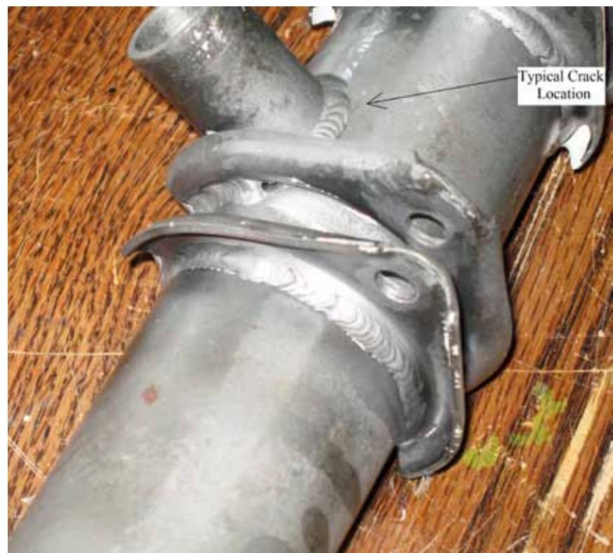
Typical crack location on a MLG torque tube.
