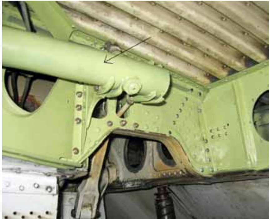
New MLG torque tube installed (along with new side brace kit).
