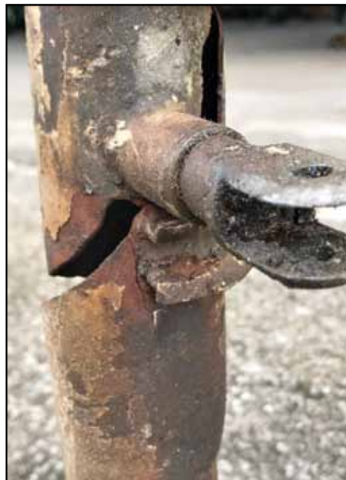
MLG torque tubes have been a known problem area for decades. In spite of a new, more robust version they can still fail. The culprit is usually corrosion which can start on the inside of the tube, making detection difficult.
