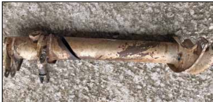
MLG torque tubes have been a known problem area for decades. In spite of a new, more robust version they can still fail. The culprit is usually corrosion which can start on the inside of the tube, making detection difficult.
