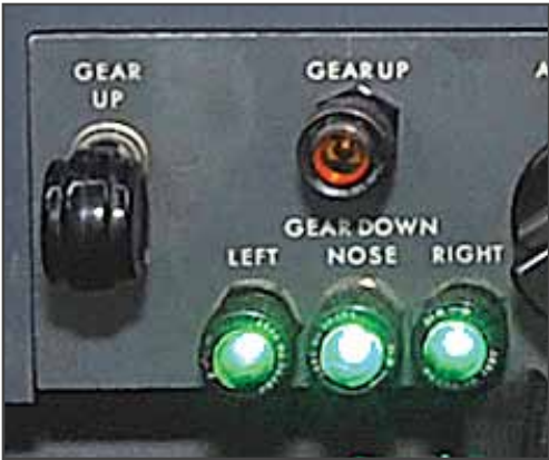
A thorough understanding of your landing gear and knowing what the panel lights mean and how they operate will make your flying safer and troubleshooting easier.
