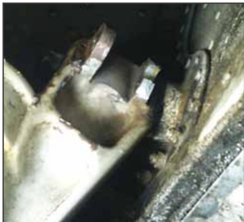
Broken ear on main landing gear upper trunion at lock link pivot bolt point.
