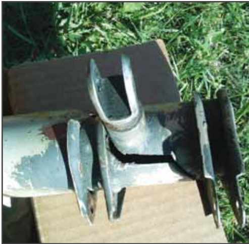
My gear incident occurred after we replaced this MLG torque tube and completely re-rigged the landing gear.
