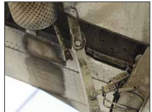
Upon landing, we surveyed the damage. Here is the broken end on the MLG outboard drive tube.
