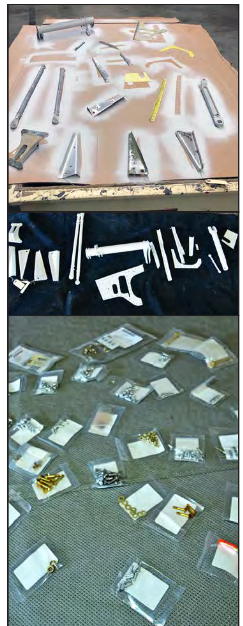
Landing gear parts and hardware. We removed, cleaned, and repainted all the parts.
