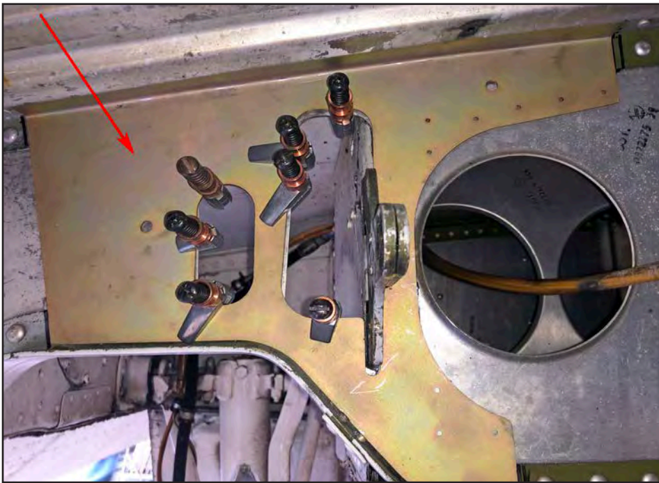
The doubler plated used for the crack repair.
