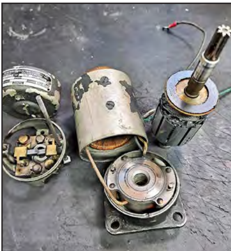
The stops on my landing gear motor were out of tolerance and the motor brake plate had glazed over. We sent it out for overhaul.
