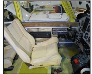
The all-important check of temporarily installed but still unupholstered interior components to closely check for proper clearance, security, and function of each component.
