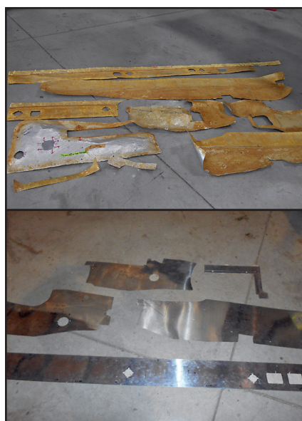
Top: Unusable set of 310R original factory side panels.
