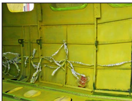
Thoroughly cleaned, corrosion-free, chromated cabin, ready for the new insulation package.
