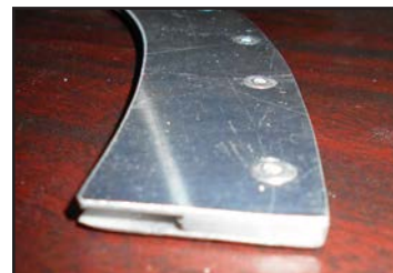
End view of the built up field-fabricated retainer strip.
