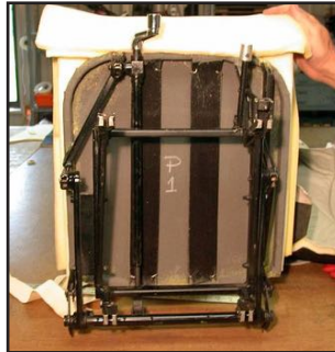
Heavy seat belt reinforcement and new heavy dacron canvas seat base sling.
