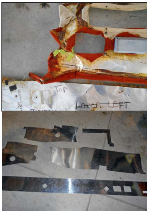
Top: Typical unusable condition of the large, very thin aluminum factory side panels found in early 310s.
