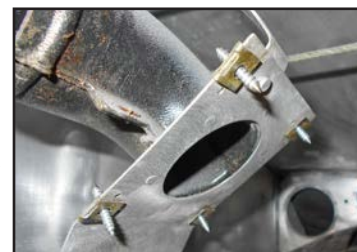
Sharpened, partially installed vent outlet mounting screws make for accurate location of holes in the new headliner.
