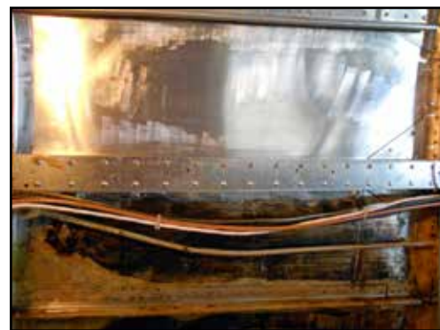
One section of a 310 cabin side skin, thoroughly cleaned with Scotch Brite and lacquer thinner.
