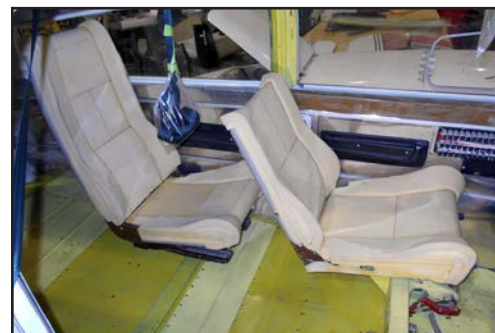
The unupholstered interior installed in order to double check everything for fit, function and clearance before it all goes into the sewing room for upholstery.
