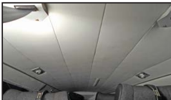
Full cabin length, multi-panel, later style Cessna twin headliner that can be mounted with either long straight rods and loops or aluminum extrusion mounting rails.
