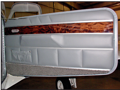
A finished door panel with hardwood inlay, rebuilt armrest and new .025" aircraft aluminum side panels, all securely held in place with nice-looking extruded aluminum divider rails.
