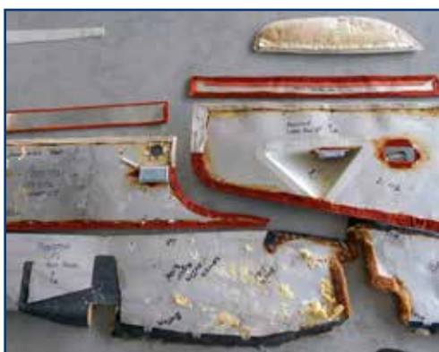
Almost every older Cessna twin will require new, more durable side panels and armrest mounts.
