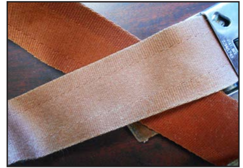
Sun faded 45-year-old Cessna lap belt.
