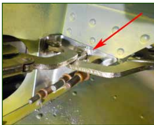
Left: Cracked pilot seat support bracket in a 310. The fix is a heavy 2024T-3 aluminum doubler.
