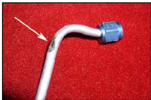
A corrosion-induced hole found in an aluminum fuel line located deep in the filthy complexity of fuel lines seen in the previous photo.
