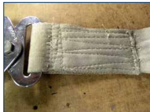
Homemade seatbelts: Note unapproved sewing and stitching pattern and absence of required certification tag.
