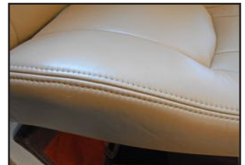
French stitch; note the exposed edges of the finish material and the top stitching thread.
