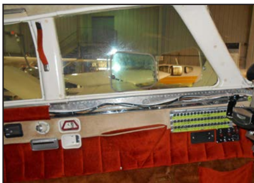
Typical plastic armrest and side panel design in a 60s Cessna twin. One large, very thin sheet of aluminum with a plastic, vacuum-formed armrest, permanently mounted by the pilot seat.
