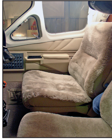
New, reinforced, aftermarket flight deck side panel armrest.
