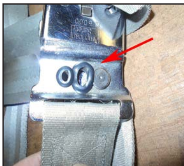
Homemade attempted fix for a worn attach fitting that employed the use of a rubber O-ring.
