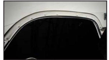
Upholstered cabin door headliner trim piece secured with #6 upholstery screws and finish washers.
