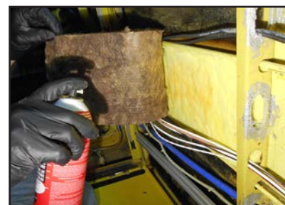
Neatly fit double layers of fiberglass insulation being lightly bonded in place with Camie 303 spray adhesive.
