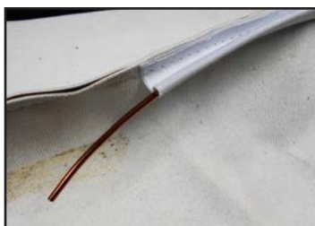
Canvas loop and bow headliner mounting system used in early Twin Cessnas.
