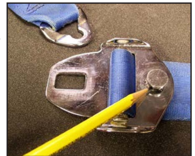
Worn nylon bushing in a shoulder harness attach fitting.
