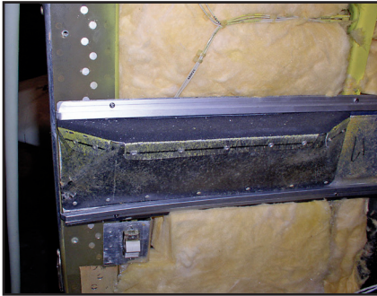
A rebuilt armrest assembly secured to the cabin side structure with sturdy extruded aluminum.
