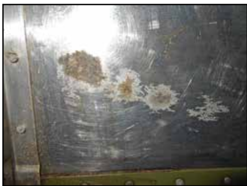
Corrosion often seen on a cabin side skin once the tar is removed.
