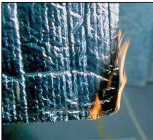
A picture is worth a thousand words: household water heater wrapping used as insulation in a 421.
