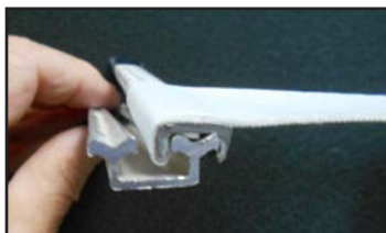
End view of the aluminum extrusion and plastic headliner mounting system (available from Recmar Products).
