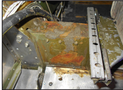
Typical corrosion-prone mess caused by gluing carpet to a spar carry through.
