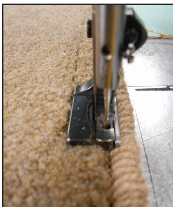
Running a 'stitch in the ditch' that permanently secures the bonded in place Velcro to the back surface of the new floor carpet.
