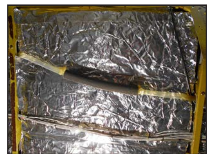
Neatly installed Sound Ex material that allows exposure of cabin plumbing and wiring.
