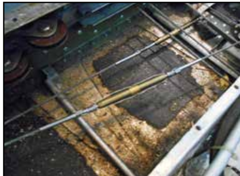
Typical oily mess found in the belly of a 40- to 50-year-old piston Twin Cessna.
