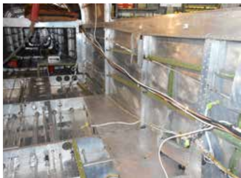
A 310 cabin, antiseptically cleaned showing partially masked wiring, cables and servos, almost ready for the application of zinc chromate.
