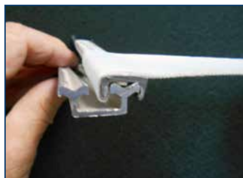
Extruded aluminum headliner retention rail system found in newer Twin Cessnas.
