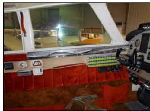
Every interior trim component shown in this photo of a 20+ year-old aftermarket interior was found to burn, including all of the cabin insulation.
