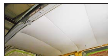
Spanwise multi-panel headliner typically installed in early Twin Cessnas.
