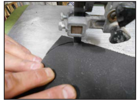
Using a band saw to quickly and neatly cut out the Sound Ex.
