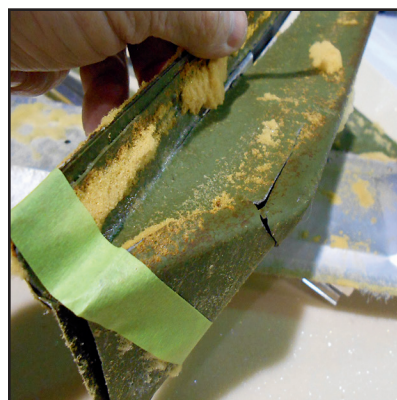
Typical damage found on plastic armrests on later-production wing mounted twin engine airplanes.
