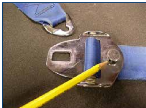
The nylon retaining sleeve that snugly holds the shoulder harness in the seatbelt buckle is often badly worn or missing, contributing to possible disconnection of the shoulder harness.
