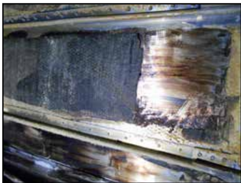
Skin damping tar partially removed by careful heating with a heat gun and scraping with a plastic scraper.
