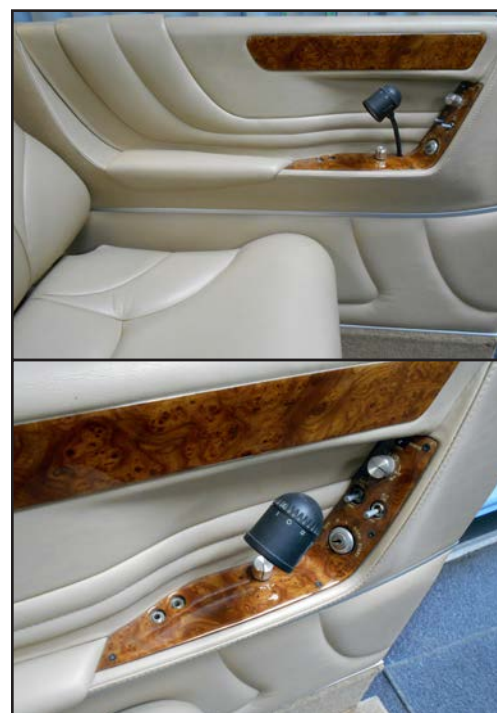
Molded fiberglass and aluminum multi piece side panels with recessed armrests and convenient, recessed accessory panel. All wood trim is high-gloss hardwood veneer.
