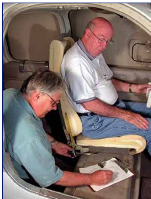
Custom fitting in a seating station to ensure correct ergonomic geometry that accommodates the physical dimensions of the pilot.
