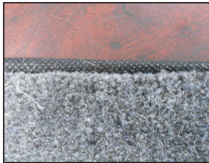
The finished product, all done with a walking foot needle feed upholstery sewing machine. No complicated and expensive carpet serger required.
