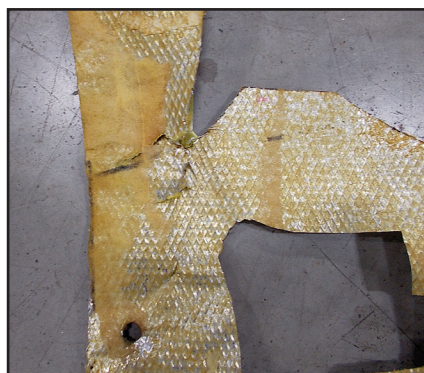
The quilting process applied to .016" aluminum didn't solve the delicate nature of original factory side panels.
