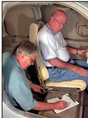
Performing an ergonomic study and recording the data allows our foam builder to create an ergonomically correct and comfortable seat.
