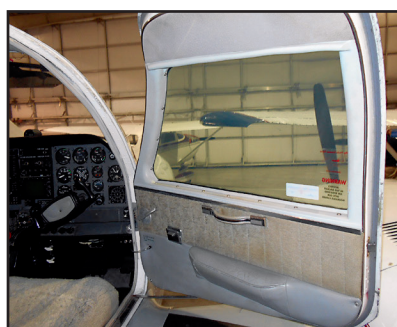
The formed stainless steel edge molding strips installed by the factory in an effort to create a pleasant looking edge closure. This tedious installation process makes it almost impossible to remove and reinstall the thin upholstery panels without damaging the panels, the stainless edge trim, or both.
