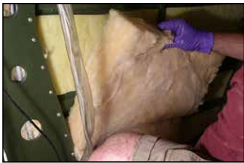
AA-approved flame retardant upholstery materials and insulation will not support the ignition or spread of a cabin fire, especially the insulation shown in this photo.
