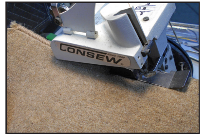
A carpet serger in action sewing a neat loop of color-matched serging thread to the edge of a new section of floor carpet.
