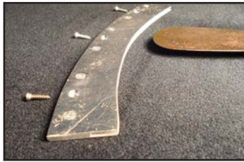
Retainer strip with 1/8" countersunk mounting holes and flush #4 sheet metal screws.
