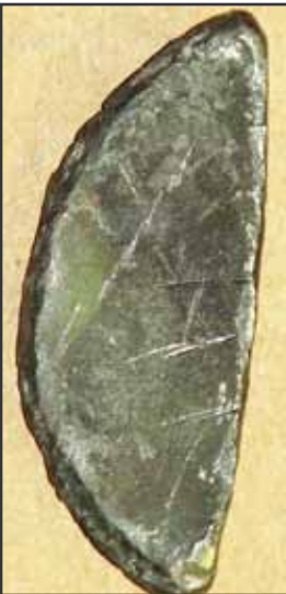
Exhaust valve piece from failure #2. We found it in the intake crossover pipe.
