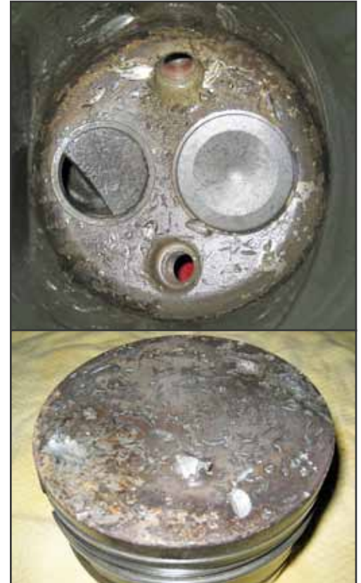
Broken valve #1 and the damage it caused before exiting the cylinder and the airplane through the exhaust system.
